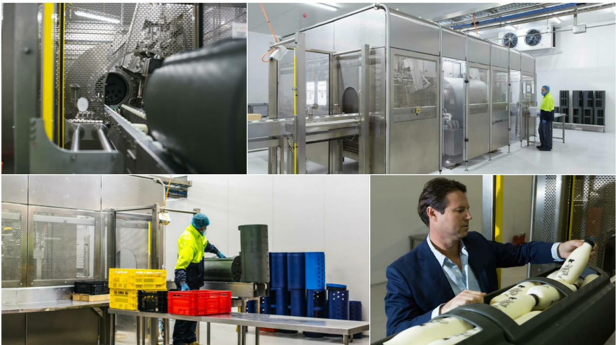
high pressure of cold water makes bottle and milk inside squash in about 15% at 7000 times atmospheric pressure to remove dangerous pathogens
